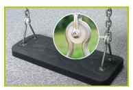
5- The swing seats are made of shock absorbing moulded honeycomb rubber. The swing chains are made of stainless steel. The seat fixing brackets are made of 10mm stainless steel wire. PVC sliding rings are fitted to limit the wear of the metal parts over time. The rings are accessed by a vandal proof, stainless steel shackle.
