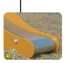
1- The sliding surface is made of stainless steel 2mm thick, shaped, bent and rolled in one piece. The side elements consist of painted panels, made of very high quality plywood with layers of birch. The colours are applied by electrostatic spraying of two-component polyurethane lacquer that is free of heavy metals, to ensure high levels of resistance to potentially aggressive chemicals such as antigraffiti cleaning products.
