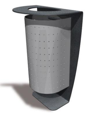
Painted steel mounting system and lid opening, thickness 8mm - painted perforated aluminium liner, thickness 3mm with 6mm rounds. Capacity 42 litres. Emptied by tipping - Lockable liner RAL 7004 - Fixing on to a concrete block
