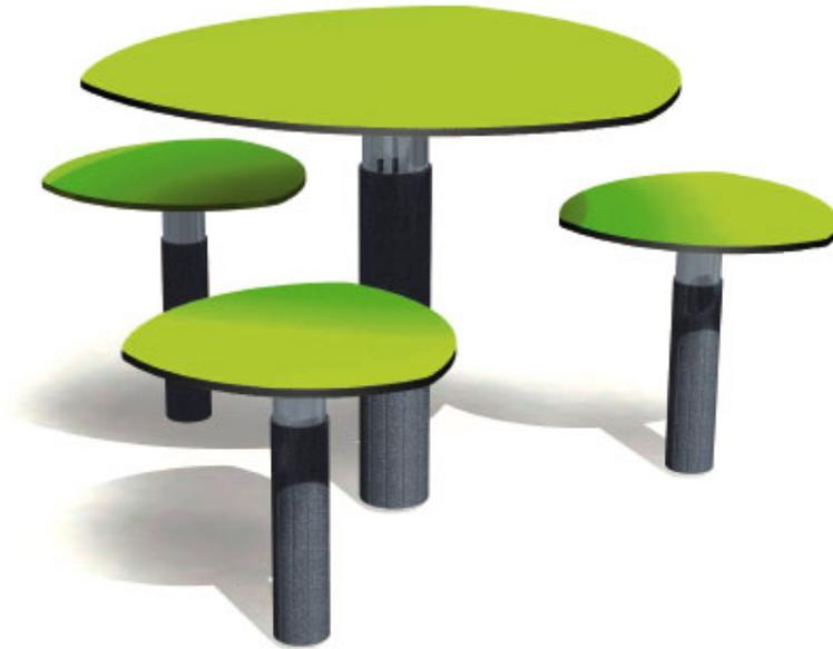
Table and seat tops manufactured from 13mm thick compact - Black polyester powdercoated steel posts for table and stools. Table: diameter 125mm, thickness 2.5mm Stool: diameter 88.9mm, thickness 2mm. Stainless steel fixings protected by ployamide anti-vandal caps
