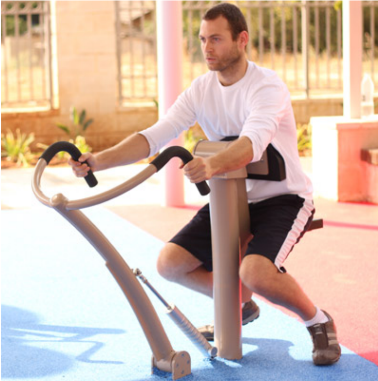
User controlled hydraulic piston
