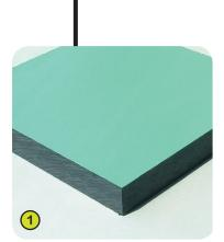
1- The coloured panels are made with a compact material 13mm thick. It is made up of 70% of softwood fibres and 30% of thermosetting resin, and it stands up to weathering very well (sun, rain, damp, etc.). The coloured surfaces are treated with products based on coloured acrylic polyurethane resins; this enables them to stand up well to UV radiation and resist damage.
