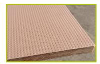
**3- The platforms** are made from a 12.5mm thick, textured, non-slip compact material (HPL).
