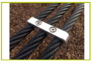
**12-The strap** is made of 3 ropes linked together with aluminium pliers. Each rope, of 16mm diameter, is made up of galvanized steel cables covered in polypropylene.
