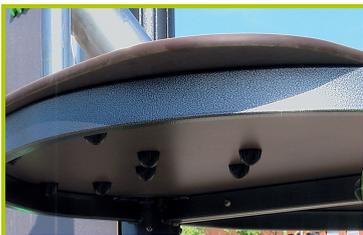
5- **The platforms** are made from a 12.5mm thick, textured, non-slip compact material (HPL). Further reinforcement is provided by lacquered galvanised steel supports, located on the underside of the platforms.
