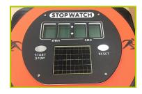
**2- The stopwatch** is machined from a polyethylene panel, embedded in a 13mm thick compact (HPL) panel. It runs on solar power. It is equipped with 2 Start and Reset buttons which are in stainless steel.
