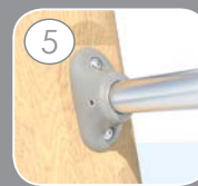
5 Fasteners and clippers made of aluminium alloys, very easy to assemble gives very stable stiff structure. Aluminium with anti-corrosive impregnation from the process of cathaphoresis, also coated with powder painting of QUALICOAT polyester paints.
