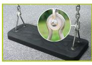
4- The swing seats are made of shock absorbing moulded honeycomb rubber. The swing chains are made of stainless steel. The seat fixing brackets are made of 10mm stainless steel wire. PVC sliding rings are fitted to limit the wear of the metal parts over time. The rings are accessed by a vandal proof, stainless steel shackle.
