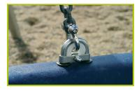
4- PVC sliding rings are fitted to limit the wear of the metal parts over time. The rings are accessed by a vandal proof, stainless steel shackle. The swing chains are made of galvanised steel.
