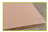
**3- The platforms and the climbing wall** are made from a 12.5mm thick textured and non-slip compact material (HPL).
