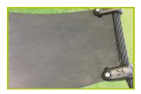
**9- The seats** are made from rubber, 13mm thick.
