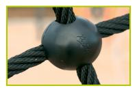
**10-The 16mm diameter ropes** are made of galvanised steel cable covered with polyester. The cables are linked together and held in place by injected polyamide spheres.
