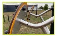
14-The stainless steel Tai Chi wheel rotation system is equipped with bearings.
