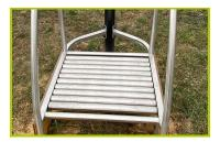
**11-The Runner rolling bars and surrounding frame structure** are made of stainless steel.
