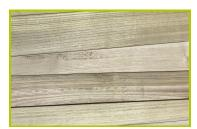
2- The boards are made from sap free robinia. The robinia is sanded and has had its bark removed. Robinia is naturally rot proof and does not require any additional chemical protection; it is equally extremely resistant to attacks from external sources (insects, fungi, climatic variations), guaranteeing the long term durability of the playground equipment.
