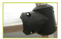
6- Injection moulded polyamide fixings connect the posts with the platforms and the various play features. They are non-toxic, flameproof and U.V. resistant. The thickness of the polyamide makes the equipement both strong and vandal resistant.
