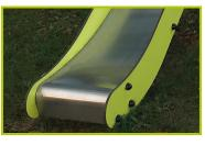
**7- The sliding surface** is made of 2mm thick stainless steel, which is shaped, bent and rolled from one piece.
