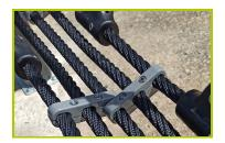
**9- The strap** is made of 5 ropes linked together with aluminium pliers. Each rope, of 16mm diameter, is made up of galvanized steel cables covered in polypropylene.
