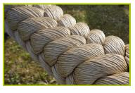
**5- The rope** is made of polypropylene.
