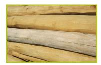
1- The different posts are made from sap free robinia. The robinia is sanded and has had its bark removed. Robinia is naturally rot proof and does not require any additional chemical protection; it is equally extremely resistant to attacks from external sources (insects, fungi, climatic variations), guaranteeing the long term durability of the playground equipment.
