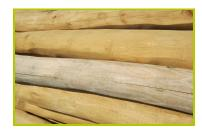
1- The 120 to 140mm diameter posts are made from sap free robinia. The robinia is sanded and has had its bark removed. Robinia is naturally rot proof and does not require any additional chemical protection; it is equally extremely resistant to attacks from external sources (insects, fungi, climatic variations), guaranteeing the long term durability of the playground equipment.
