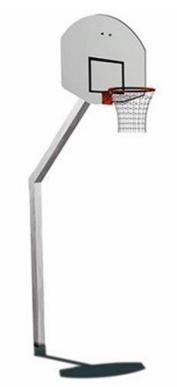
Reinforced fibreglass board with a reinforced basket. Frame made of 100mm cross-section square tube, with epoxy lacquer. Board size: 1.20x0.90m - Hoop height: 3.05m
