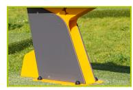
**3- The structure of the equipment** is made of painted galvanised steel. The coloured panels are made from a 13mm thick compact material (HPL). Robust in construction, it has excellent weather and vandal resistance properties.
