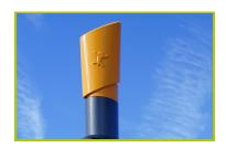
1- The 102mm diameter posts are made of painted galvanised steel. The grained finish has a slightly undulating surface for increased scratch resistance. The caps are made of rotary moulded polyethylene.
