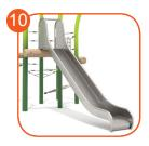
Slide made of stainless steel AISI 304. The metal sheet is 2 mm thick and the end section is finished with a band made of pipe 33,7 mm.
