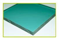
**21-The portholes** are made from 8mm thick methacrylate (PMMA).
