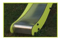
**16-The sliding surface** is made of 2mm thick stainless steel, which is shaped, bent and rolled from one piece.
