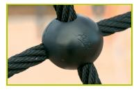
**4- The 16mm diameter ropes** are made of galvanised steel cable covered with polyester. The cables are linked together and held in place by injected polyamide spheres.
