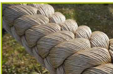
**9- The rope** is made of polypropylene.
